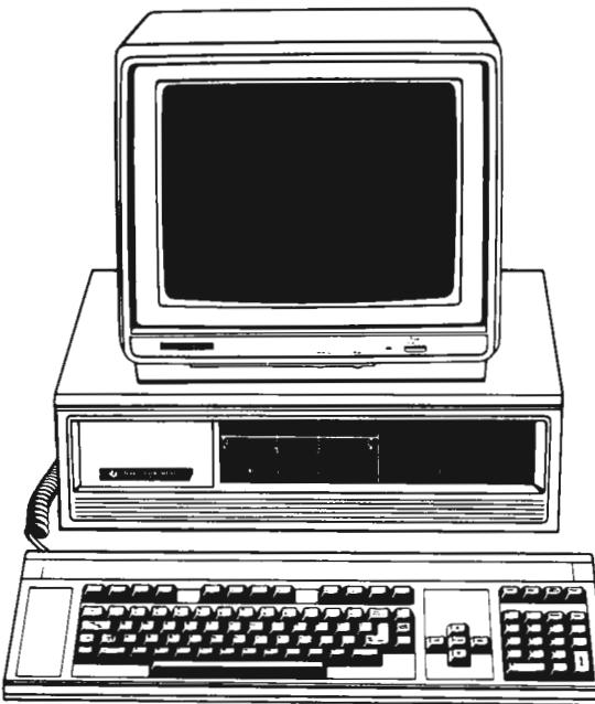
memory and 320K diskette mass storage. Add up to 768K RAM internal memory, a 10-megabyte internal Winchester disk drive and two internal communications modems.
