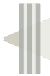
Reinforced concrete loss: 40 to 90%
