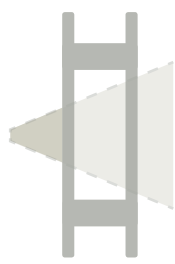
Wood, plaster walls loss: 5 to 20%
