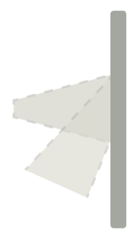
Enclosure in metal loss: 90 to 100%
