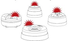
When all alarms flash the red LED, they are connected and can be switched out of 'Learn Mode' and installed.
