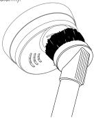
**NOTE**: You can easily vacuum clean the smoke chamber through the dedicated openings in the top cover, and it's possible to test the alarms by pressing the cover at the same time.
