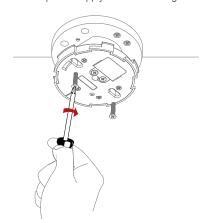
Once the mounting base with power supply is installed, attach the alarm by twisting clockwise until it clicks. If the battery is either missing or inserted incorrectly, the smoke alarm will not be able to click into the mounting base.
