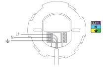
Connect the 3 wires to the power supply: Live feed (L1), neutral (N), Ground  $(\bot)$ .
