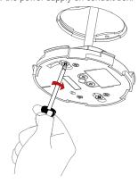
**NOTE**: Mounting base is not used when the alarm is installed on conduit box.
