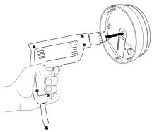
Install the power supply into the mounting base ring or use the conduit box as shown in option 1 & 2.
