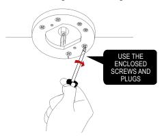
Screw the power supply on the mounting base.
