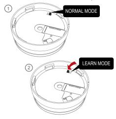
Please note: The learn switch placed on the back of the alarm can only be in learn position when the alarm is disassembled from the power supply unit. The learn switch will automatically switch to normal position when the alarm head is fitted to the power supply.
