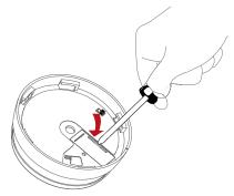
Replace the battery respecting the polarities. Attach the alarm on power supply by twisting clockwise until it clicks, and test the alarm.
