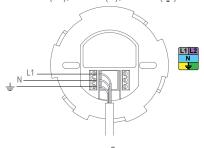
Screw the power supply on conduit box.
