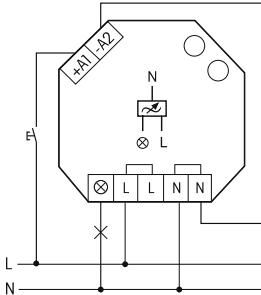
Control voltage, supply voltage and switching voltage 230V
