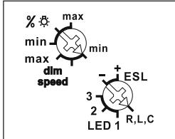
With the top rotary switch %\* dim speed can be adjusted either the minimum brightness level (completely dimmed down) or the dim speed.
