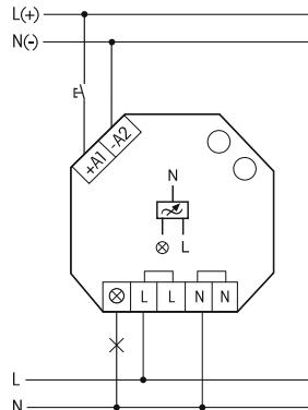
Universal control voltage 8..230V UC, supply voltage and switching voltage 230V
