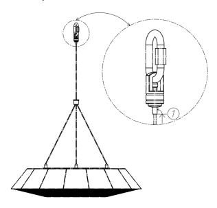
Step 2: Unscrew the hook nut in direction of arrow.
