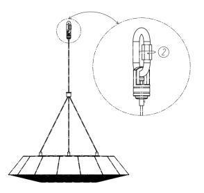
Step 3: Tighten the nut in direction of rotation arrow.
