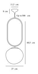
Voltage (V): 230 Volt IP degree if the fixture includes two types of IP degree: IP20 Maximum compatible bulb wattage (W): 15W Class (Class I, Class II, Class III): Class 2 (Double isolated) Lampholder type (eg, E27/E14, etc): E27
