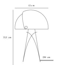
Voltage (V): 230 Volt IP degree if the fixture includes two types of IP degree: IP20 Maximum compatible bulb wattage (W): 25W Class (Class I, Class II, Class III): Class 2 (Double isolated) Lampholder type (eg, E27/E14, etc): E27
