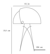
Voltage (V): 230 Volt IP degree if the fixture includes two types of IP degree: IP20 Maximum compatible bulb wattage (W): 25W Class (Class I, Class II, Class III): Class 2 (Double isolated) Lampholder type (eg, E27/E14, etc): E27
