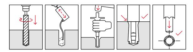
Instructions on inserting the anchors
