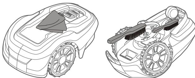
**WARNING! Press the STOP button and remove the safety key before cleaning.**
