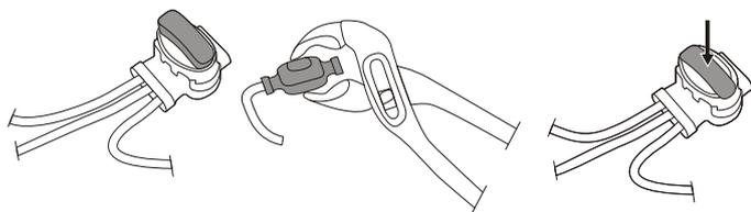
If the boundary wire is too short, use provided splice and guide wire connectors to splice additional boundary wire as follows:
