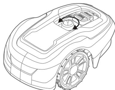
For the first few weeks of mowing, set the cutting height to 60 mm to avoid cutting the boundary wire and guide wire. Lower the setting one step each week thereafter until the desired cutting height is reached.
