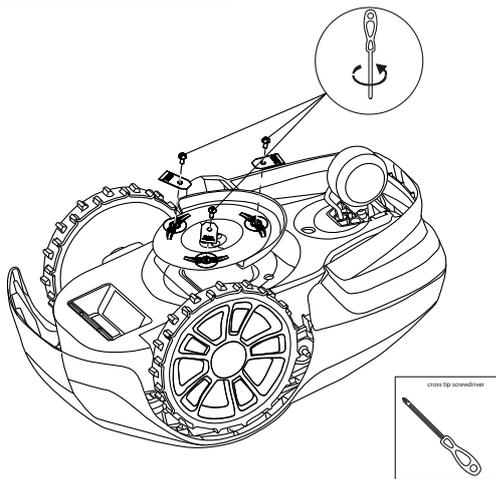
**WARNING!** Press the **STOP** button and remove the safety key before replacing blades and wear protective gloves.
