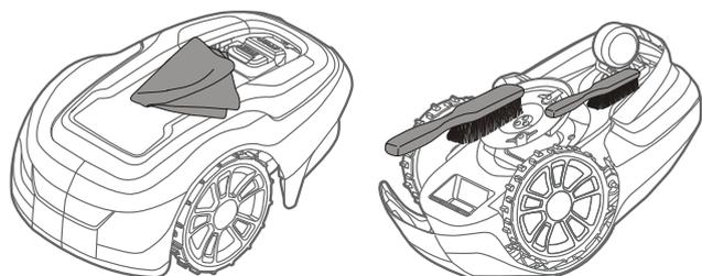
**WARNING! Press the STOP button and remove the safety key before cleaning.**
