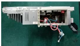
2) Disassemble lead wire connected with terminal board.(5 pcs)
