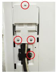
3) Loose the screws, remove the connecting cable from Terminal Board.
