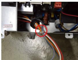
2) Remove the screw, then remove the Terminal Board.
