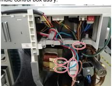
(Disassemble the control box ass'y)
