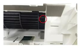
23) Hold and press the Cross Flow Fan to left side as much as possible, meanwhile, take Fan Motor out.
