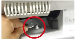
19) Remove the screw of Bracket, and take Bracket out.
