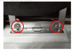
13) Unscrew the nut, take out the Propeller Fan carefully.
