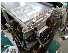
11) Cut the wire fixing band fixing the transfer connector of the compressor and control box ass'y, then disassemble the terminal of reactor and compressor, after all, disassemble control box ass'y.
