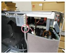
10) Pull down the terminals connecting the electric box substrate. Take out the thermistor lead wire from guide groove.
