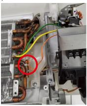
14) Use a pincer to press the 4 spacer into the Control Angle to remove the PWB.
