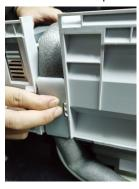
27) Enlarge the angle between Tube Ass'y and Cabinet. Then take the Evaporator out.
