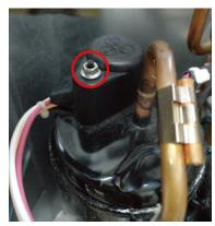
10) Disconnect three terminals on the Compressor.
