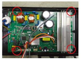
Note: Before changing control board, the workmen should wear anti-eletrostatic gloves.
