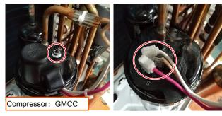
16) Disassemble thermistors(4 pieces) and thermistor clamps(1 piece) .
