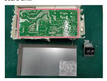
(Disassemble 7 screws on control board unit.)
