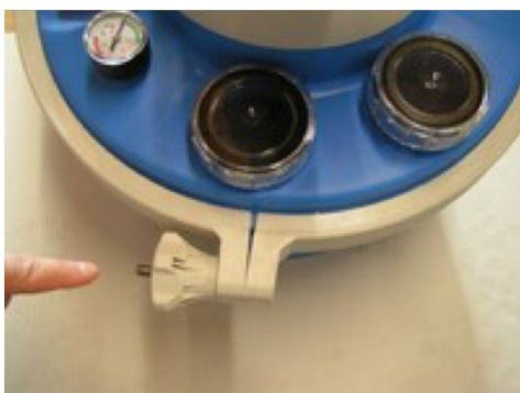
Photo 4.1a - A plastic clamp is included for tightening the pressing ring.
