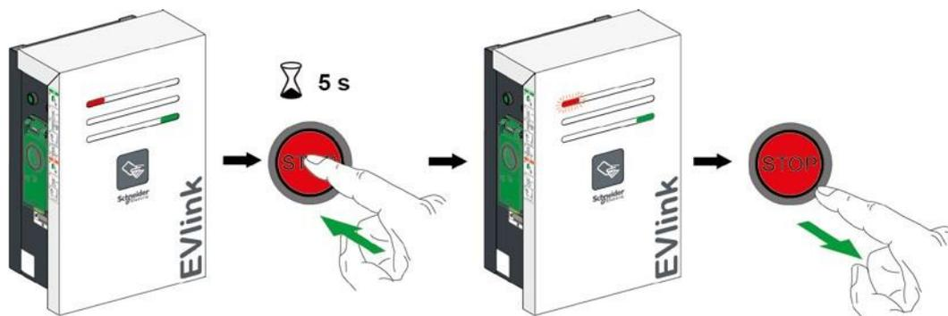
Note: Press the stop button on the fault side.
