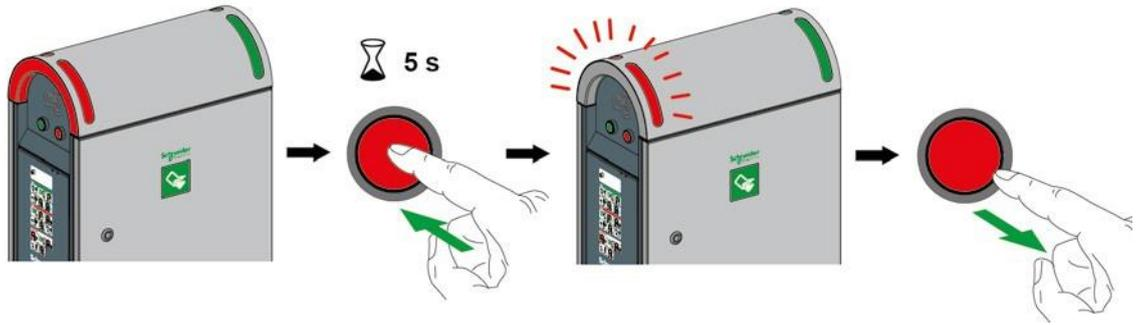
Note: Press the stop button on the fault side.
