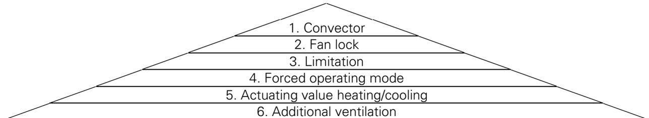
The *heating system = convector / fan coil* and *cooling system = convector / fan coil* parameters have the highest priority (1.). The fan is not actuated with the convector.
