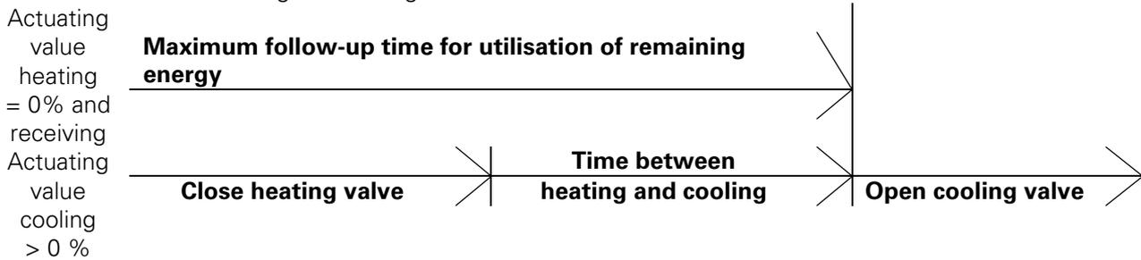
Transition between cooling and heating.
