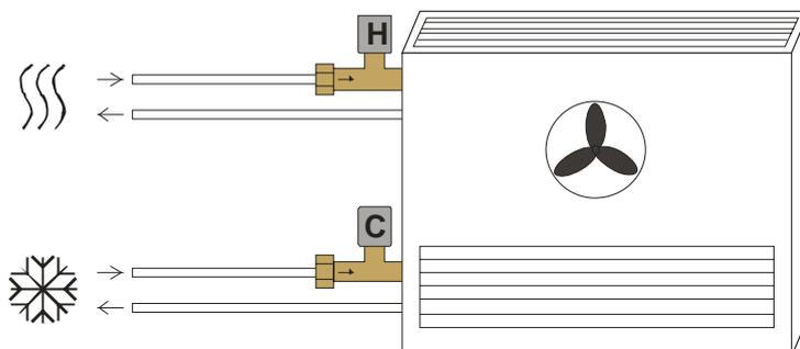
When used in a 4-pipe heating/cooling system the heating valve is connected to the *V1* terminals and the cooling valve to the *V2* terminals.
