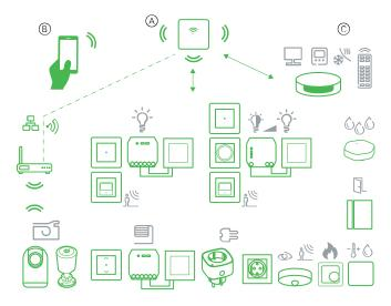
The Wiser gateway (see A) is the center of the system, processing control requests and status reports for connected Wiser devices.
