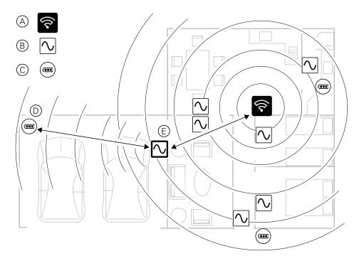
**TIP:** The battery-powered motion sensor in the garage (D) is a long way from the gateway. However, the sensor can connect to the gateway via the mainspowered device being used as the garage light switch (E). This is because mains-powered devices also act as system network extenders. Consider this when deciding where to locate the gateway.
