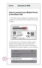
After successfully connecting the phone to Wi-Fi, go back to the App. When the connection is progressed, the AP mode commissioning is successfully completed. Tap **Done** to finish.
