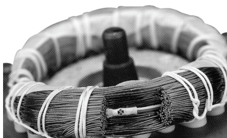
PTC sensor incorporated in windings
