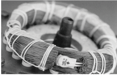
Thermal switch incorporated in windings
