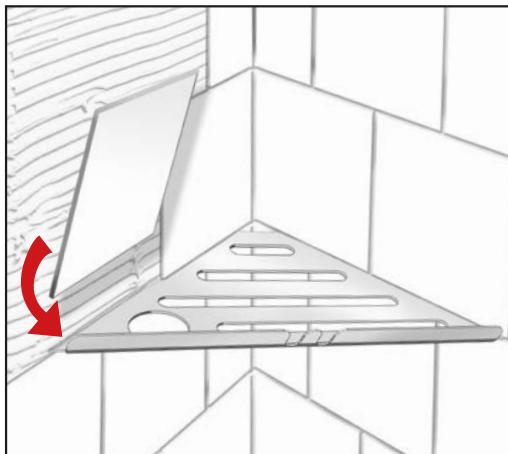
(UK) The corner shelf is attached between two tiles during tiling.
