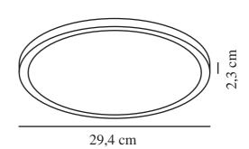
Voltage (V): 220-240 Volt IP degree: IP20 Class (Class 1, Class 2, Class 3): Class 2 (Double isolated) Socket type: LED Module Parallel connection: False
