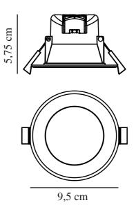
Voltage (V): 230 Volt IP degree: IP20 Class (Class 1, Class 2, Class 3): Class 2 (Double isolated) Socket type: LED Module
