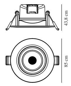
Voltage (V): 220-240 Volt IP degree: IP23 Class (Class 1, Class 2, Class 3): Class 2 (Double isolated) Socket type: LED Module Dimmerable: True Parallel connection: True
