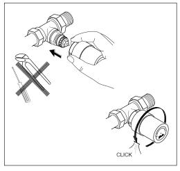
The knob snaps onto the valve eliminating the need for any mounting tool.
