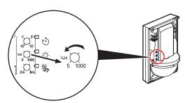
In order for the sensor to detect only when it is dark, turn the screw (potentiometer) counterclockwise.
