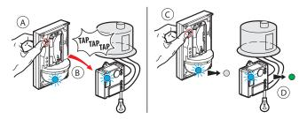
Phase A : Press the ON button on the wireless switch you wish to pair, while tapping it three times onto the micromodule you wish to control.
