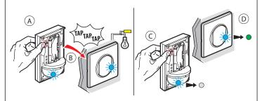
Phase A: Press the ON button on the wireless switch you wish to pair, while tapping it three times onto the light switch you wish to control.
