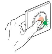
To complete your installation, briefly press the middle of the wireless master switch. All the indicator lights on the products switch off.
