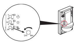
To reduce the sensitivity of the motion sensor, turn the screw (potentiometer) counterclockwise. The detection will then be at a shorter distance.
