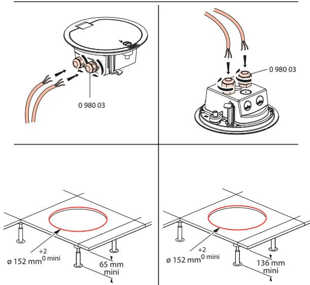
(2) Drill the back of the box at the right diameter according to the cable gland (max Ø 20 mm). The cable gland had to be well adapted to the cable. Introduce the cables in the cable gland.
