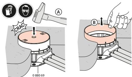
3) Drill the back of the floor box at 20mm (A) and add the cable protection (B)
