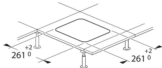
Floor space dimension of the box (*cover's* dimensions) = 283x283mm
