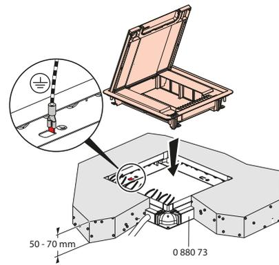
Cover can be removed for an easy installation of socket
