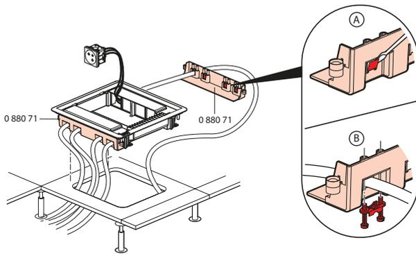
Cable retainer function can be used only with cables (A & B).
