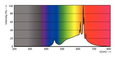
Spectral Power Distribution Colour - MAS LEDCandleDT2.5-25W E14 B35 CL G
