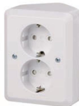
The corner-mounted Jussi 2512H.13 is a surface mounting box for two 1-gang Jussi devices, including controllers, fault current guards and other equipment requiring plenty of installation space. It can be installed both vertically and horizontally. A standard 85 mm 2-gang cover frame 2512 is used with the box. The protection class is IP20.
