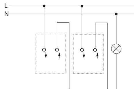
Watchdog Standard 180 is intended for direct controlling of incandescent lamps and electronic transformers. Other use of device will damage the it and may cause danger. When several Standard devices are parallel connected the minimum load will change: 1 pcs 40 W, 2 pcs 75 W, 3 pcs 100 W and 4 pcs 200 W.
