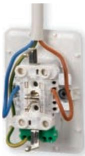
The surface mounted 2-gang Jussi socket outlet has been renewed inside. The new insert is safe, as the shutters are integrated in the insert. The insert is also smaller and the wires are connected from the front in a 60° angle.
