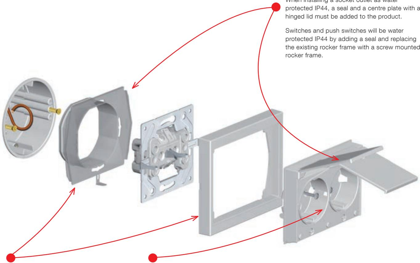
Seal 2463 is used with 85 mm cover frames and seal 2464 with 100 mm cover frames in water protected IP44 solutions.
