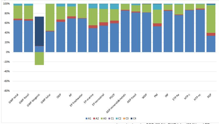
Above results highlight that module A1 (extraction and provision of the raw materials) is the one characterized by the most part of the environmental impacts with an average incidence of 64 % (values varying between 12 % and 88 %). The second largest contribution to the total impacts comes from module A3, with an average incidence of 23 % (values varying between -26 % and 58 %), where manufacturing processes dominate the
