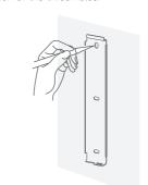
2. Drill three holes (φ6) in the wall according to the marks. Put expansion screws into the holes.
