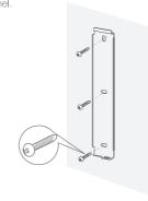
4. Choose an appropriate angle. Put the upper slot (at the back of the unit)down into the upper hook (at the mounting panel). Make the dispenserfit tightly to the mounting panel. Push the dispenser slightly down to make sure both hooks be put in the slot well. Then use hex key to lock the anti-
