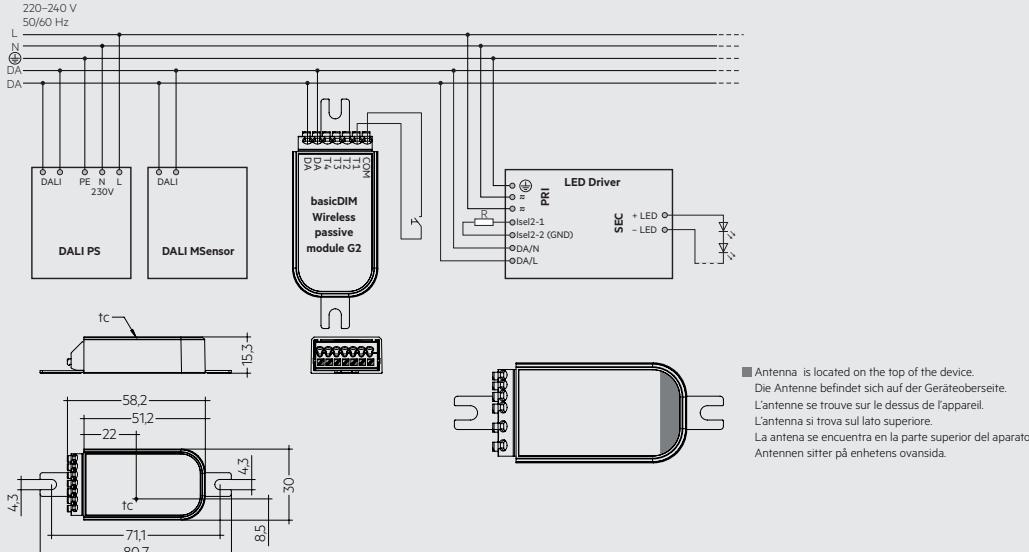
**UK** The basicDIM Wireless passive module G2 is a Bluetooth® DALI controller with 4 freely configurable push-button inputs. The module is powered by the DALI bus, no additional mains supply is needed.
