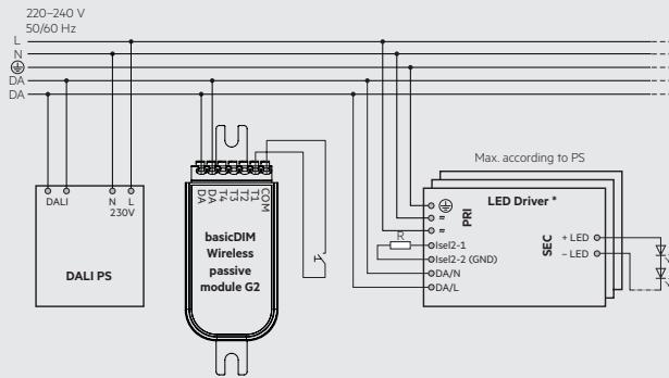
\* Max. 4 DALI single / group addresses (A0 ... A3 / G0 ... G3) controllable, depending on the device profile of the basicDIM Wireless module.
