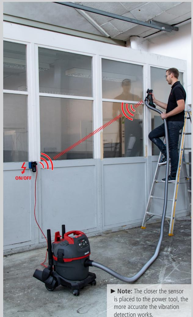
► **Note:** The closer the sensor is placed to the power tool, the more accurate the vibration detection works.
