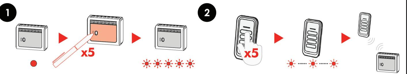
NB: The connection of the transmitter to the receiver can take between 5 and 15 seconds
