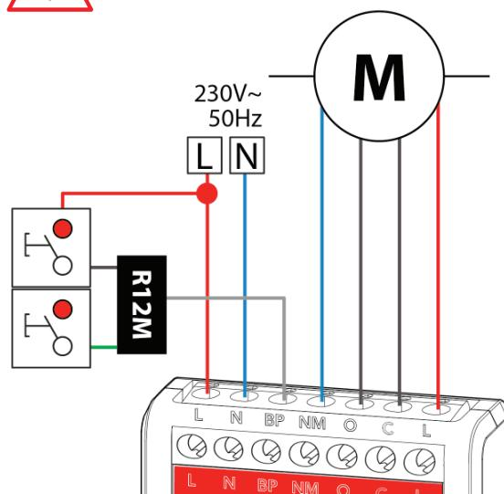
By using the R12M accessory with double push-button, I will have that the green wire of the R12M will only send the closing command, while the brown wire will only send the opening command.
