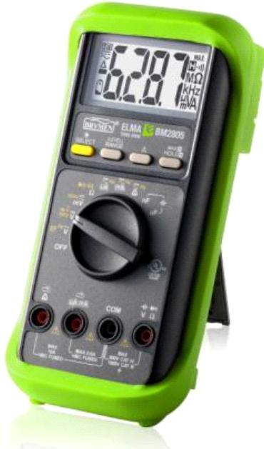
Elma BM2805 is a sturdy TRMS multimeter with backlit LED display capable of measuring voltage, current, frequency, resistance, capacitance, diodes and continuity. Functions include max-hold, data-hold, auto-range, relative values and VFD filter.
