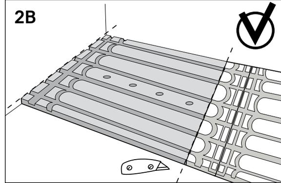
(Figure 3) Cut out a channel for the flexible floor conduit connected to the sensor for the floor heating thermostat. Then cut out a 10x30 cm square that is only 1 cm deep. The sensor will be placed here.
