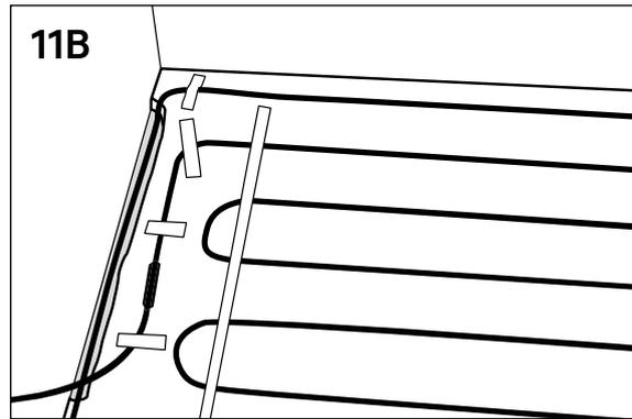
(Figure 12) If there is heating cable in all the outer grooves, make a cut out in the board all the way to the floor and place any excess cable here.
