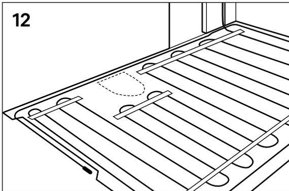
(Figure 13) Tape new strips of tape parallel with the first strips using about 6 strips every metre.
