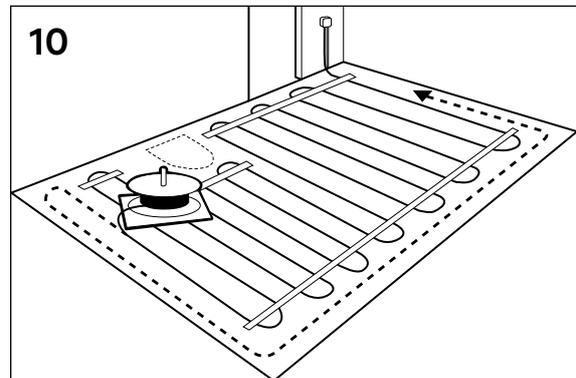
(Figure 11A+B) If you have to overlap the connection cable to get to an empty groove: Cut out a 20 mm wide channel by the wall all the way to the concrete subfloor and run the heating cable through.
