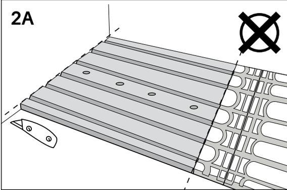
**Wet areas** Do not lay the Cable Board in a shower area where there are inclines to floor drains. We recommend instead using the Ebeco Thermo Board (89 601 60) for this area. Install the Thermo Board according to the supplied instructions. The cable is laid directly on the Thermo Board as instructed.
