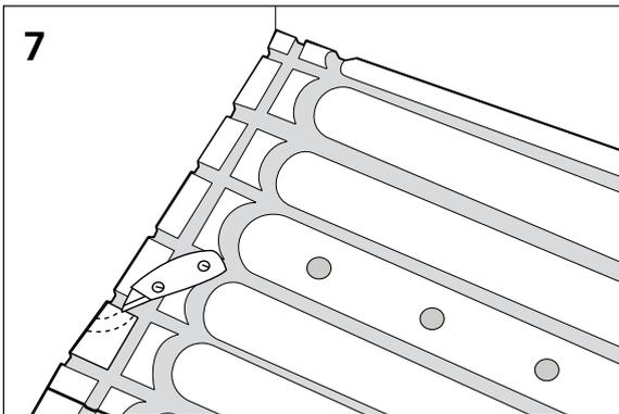
(Figure 8) Place the connection cable in the groove and draw it the closest corner. Tape the cable in place in the wider groove at the board's short edge and leave the tape roll in place. Run the cable along the next outermost groove and continue towards the opposite wall.
