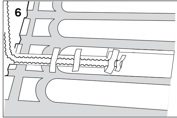
(Figure 7) Cut out a small space in the board so that the connection cable can be drawn to the outer groove in the board.
