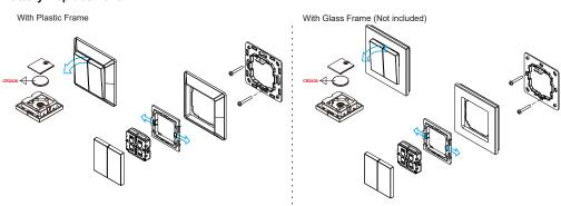
The key part of this controller is a universal, extremely rotary standard switch element that can be integrated in numerous frames by different manufactures as below list:
