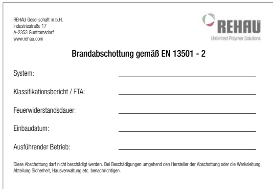
Fig. 11-2 Identification plate of the fire protection system
