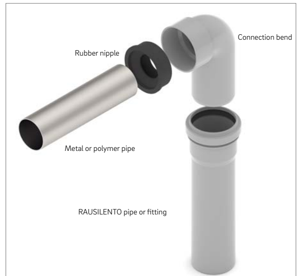
Fig. 08-6 Installation of RAUSILENTO waste tap elbow
