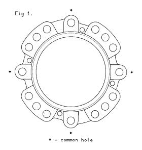
MaxiDaptors have flange configurations as shown in Fig. 1. This configuration is combined PN10 and PN16. To assemble against mating flange, locate the four common holes first, the remaining holes will then align with their respective mating flange holes.
