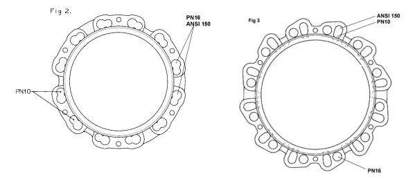
MaxiDaptors have flange configurations as shown in Figs. 2 & 3. These flanges can be bolted to PN10, PN16 or ANSI Class 150 flanges. Connect the MaxiDaptor to the other flange using the appropriate flange bolt holes.
