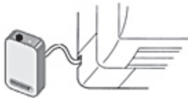
Figure 4.- IntesisHome® device and AC placement
