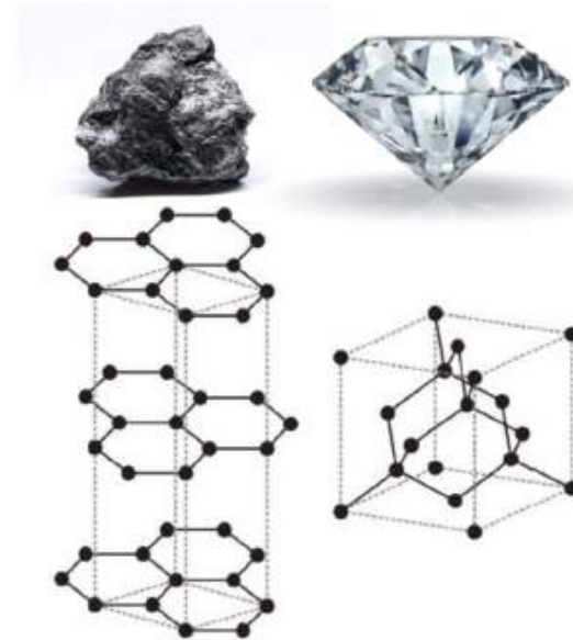
Figure 1: Graphite ( sp^2 ) and diamond ( sp^3 ) structure
