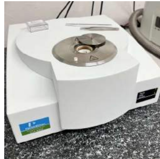
PerkinElmer TGA 4000 coupled with PolyScience chiller
