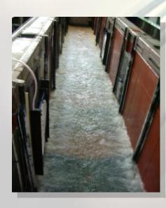
Suction hoods alongside the tank made in polypropylene and complete with setting panels on the suction holes
