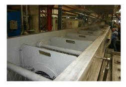
The first **electrolytic pickling** tunnel produced in Italy, has been operating at Marcegaglia Forlì for some years already. In the developing process of the Company it represents an important part for the reduction expensive handling of the operations of the bundles.
