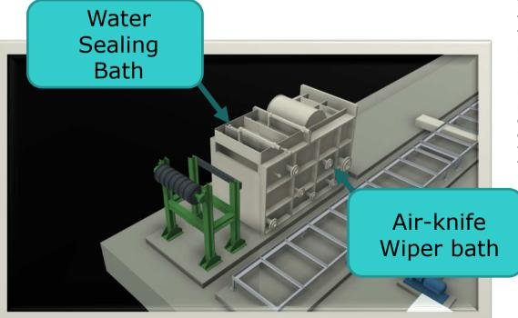
The water-veil traps are installed to prevent the escape of vapour from the pickle liquor. The water is pumped inside the sealing system by pumps; those pumps are installed on the rear side of the machine and connected by flexible pipes. In case of pump fault, a diaphragm valve will automatically open assuring the continuity of the veils with the industrial water from factory distribution pipe.
