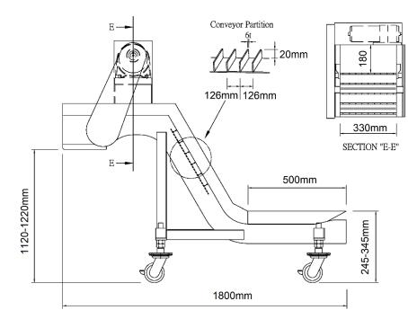
HSI Transporting Conveyors are designed to move a variety of materials from process to process. Steel belt and cleat materials are ideal for conveying small parts efficiently.
