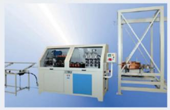
order to straighten and cut tubes with diameters from 8 up to 25 mm, and complex profiles with similar section.
