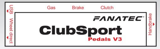
IMPORTANT: Connect the ClubSport Pedals either by USB cable OR by RJ12 cable to a wheel (base). Never connect both ways in parallel to avoid hardware damages!
