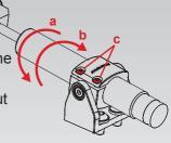
Now you can check the damper effect by pressing the pedal with attached and fixed ClubSport Pedals V3 Damper Kit. During that you can change the damper adjustment by turning the knurled plate at the back end of the damper, see picture below:
