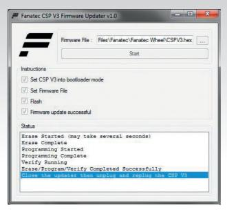
IMPORTANT: The ClubSport Pedals V3 is secured by firmware and by driver so that usually it is not possible to install wrong firmware files on the ClubSport Pedals V3! Do not try to force installation of any wrong firmware to the ClubSport Pedals V3 to avoid damages.
