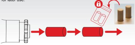
Insert the small Polyurethane spring (E) from Brake Performance Kit package content into the preload screw:
