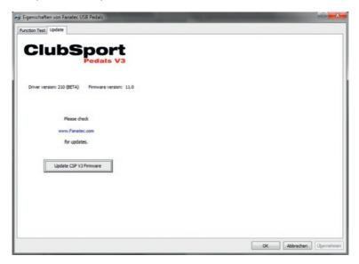
This page gives you detailed informations about the currently installed PC driver version and the currently installed ClubSport Pedals V3 firmware version. There is also the button 'Update CSP V3 Firmware', see chapter 'Firmware update procedure' of this manual for more detailed information about the firmware update process itself.
