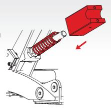
Attach the Pedalbox onto the pedal rod and hang it back into the lower stroke.
