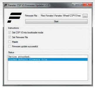
Now the user has the opportunity to select a different ClubSport Pedals V3 firmware file than the default selected file by pressing the button with the three dots if necessary. Usually the latest PC driver version already includes the latest ClubSport Pedals V3 firmware so this step is not necessary for the user.
