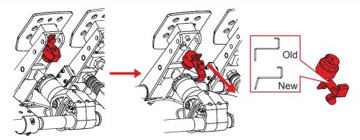
Attach the rumble motor upside down with the new rumble motor bracket:
