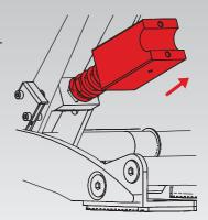
Attach the new spring with corresponding spring guides onto the pedal rod.
