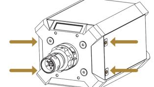
Turn the locking ring in a CW direction to the back of the shaft. Make sure the rubber ring is not compressed.
