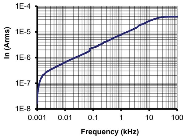
Figure 14: Typical total output current noise (rms) with  $R_M = 50 \Omega$
