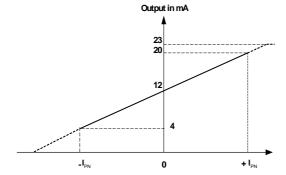
Note: 1) The performance specified in the datasheet is valid within the 4-20 mA output range only.
