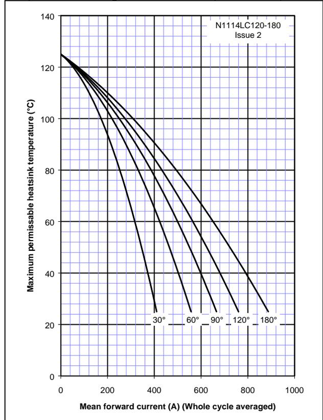
Figure 7 - On-state current vs. Power dissipation - Single Side Cooled (Square wave)
