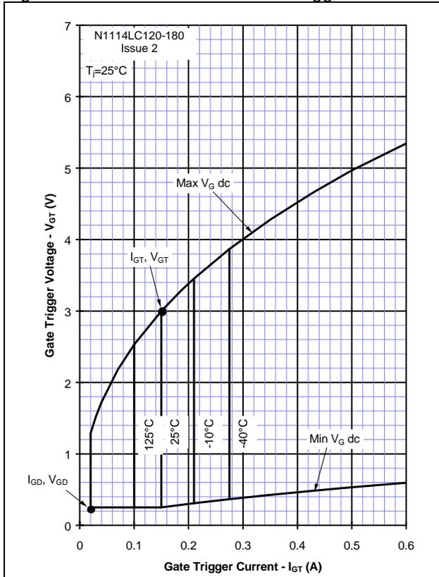
Figure 12 - Gate Characteristics - Power Curves
